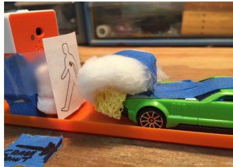
Modified Bumper (Top) using pieces of dish sponge
