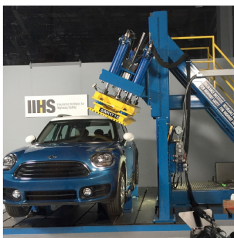
Figure 2. IIHS Roof Strength Test
