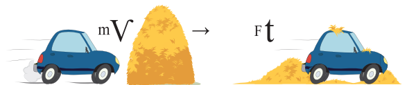
Figure 1. Stop the truck with a small impact force applied over a long time (i.e. truck hits a haystack and gradually slows to a stop with very little damage)
