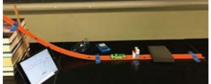
Figure 1- Crash Test Track Set-Up Height of starting line above table (cm) = 23 cm
