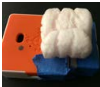
Figure 5 - Packing peanut attached to sensor
