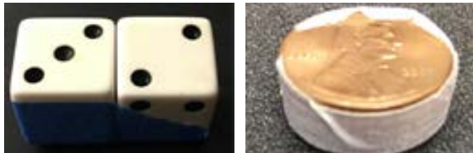
Figure 2 - Sensor base (Left) Two dice or (Right) four pennies
